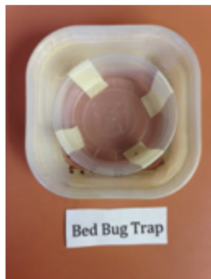
Figure 6. The small container has been glued inside the center of the large container. The walls of the containers should not touch.
