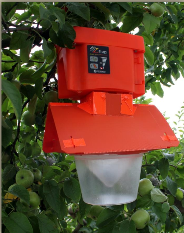
Z-Trap electronic insect trapping device Image Credit: Purdue University, Purdue Research Park
